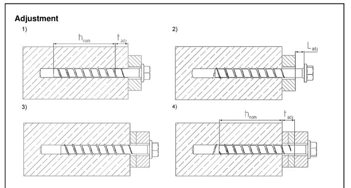
It is permissible to untighten the screw up to two times for adjustment purposes. Therefore the screw may be untightened to a maximum of  $L_{adj} = 20$  mm to the surface of the initial fixture.
